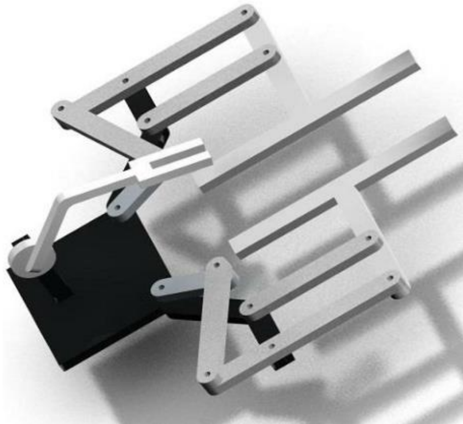
Figure 4.3: Gripper (Final Design) – With parallel link mechanism
