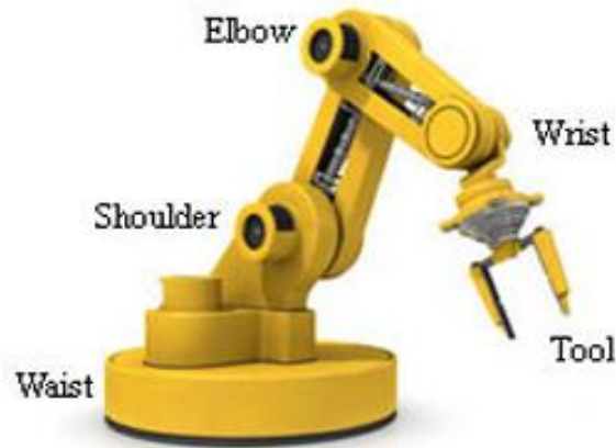
Figure 3.1: Parts of a Robotic Manipulator
