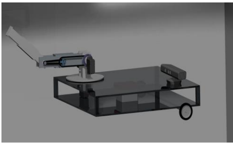
(a) Mobile robot platform with Kinect on the top
