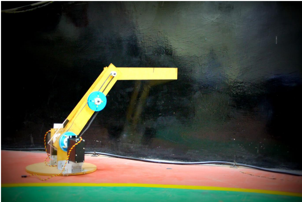
Figure 5.3: Arm assembly (without platform and gripper)
